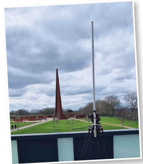
The antenna for RAF Waddington Amateur Radio Club's ADS-B/ACARS station.
